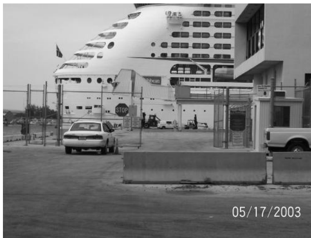
FIGURE 8.6 Temporary concrete barrier. Barrier systems provide flexibility and enhance physical security when managing access into restricted areas.
