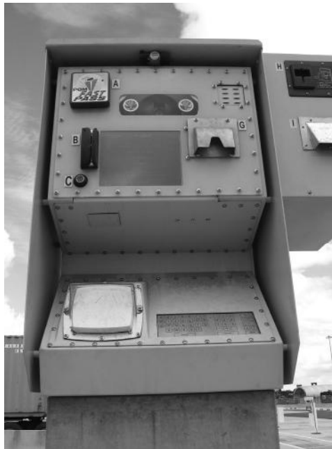
FIGURE 12.2 Automated gate pedestal at cargo entry processing facility enables truck drivers to interact with both port security and business processing systems without the need for physical person-to-person transactions.
